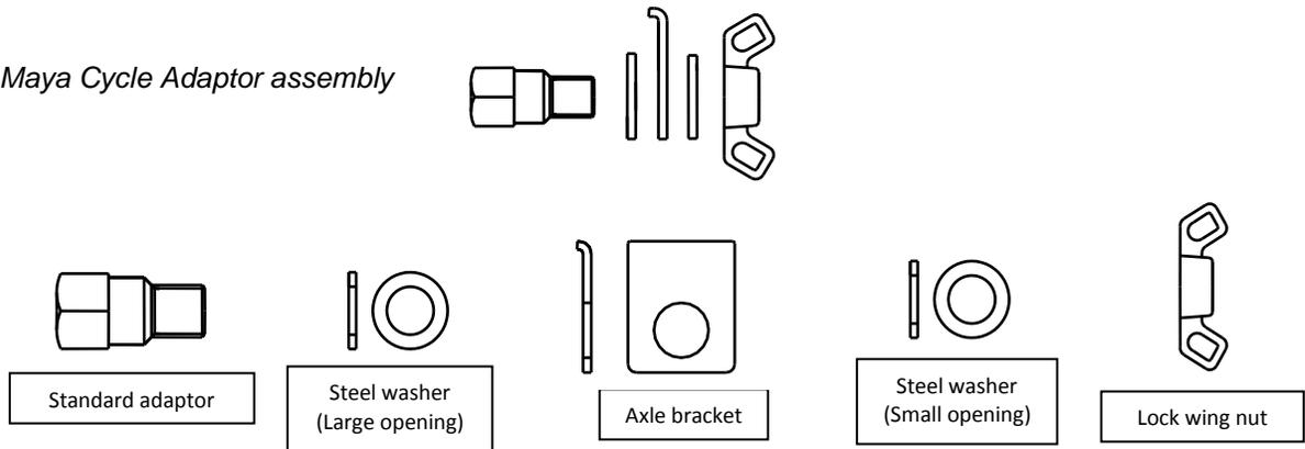
Figure 2 Maya Cycle Quick Release skewer assembly
